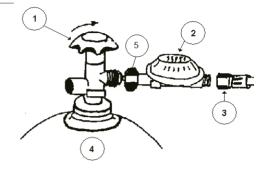
Every time a newly filled gas bottle is connected, a new rubber washer must be fitted. In most cases, your gas supplier will include it with the bottle.
